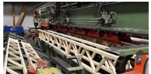
Manufactured in a 100% robotic process, TRIFORCE® joists are also individually tested beyond their load capacity, ensuring unmatched quality and reliability, an important aspect as per Bonneville Homes' R3000 quality program.
