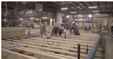
The prefab home manufacturer installs plumbing, electricals and HVAC before the house leaves the factory, accelerating onsite completion. Hiding mechanicals in the floor cavity also makes the home more spacious and can allow more storage space.
